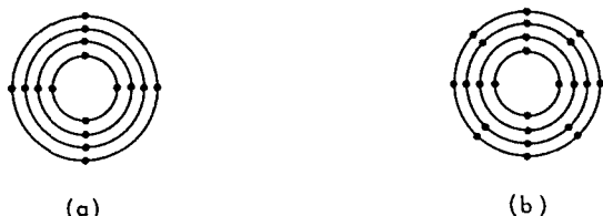
FIGURE 10-17. Disks with (a) the same number of bits on every track and (b) more bits on tracks in an outer zone than on tracks in an inner zone.
